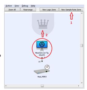
You select one of the devices in the group to be the Master and place it on the crown at the upper center of the zone (the Master zone). We will use the MassCore in the example here.
